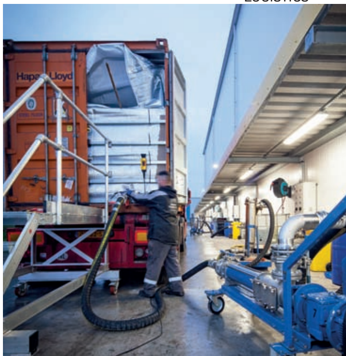
MOST OF THE RUBBER LATEX ARRIVES AT THE TERMINAL IN 20FT CONTAINERS. EACH CONTAINER HAS A PPE BAG THAT CAN CONTAIN 23,000L OF RUBBER.
